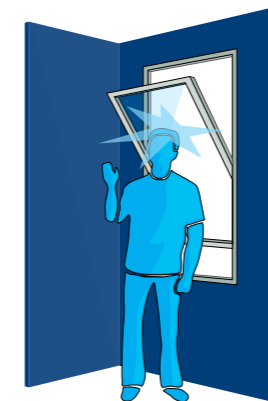
Risk of injury caused by sash impact.
